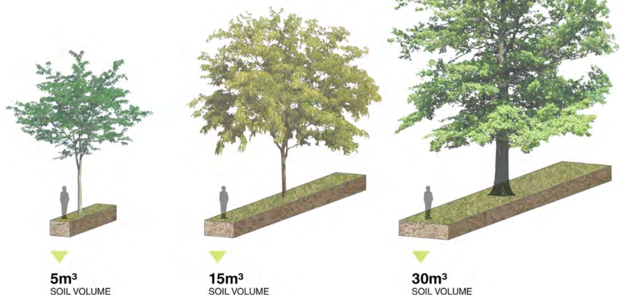
Diagram illustrating the relationship between uncompacted soil volume and tree size
