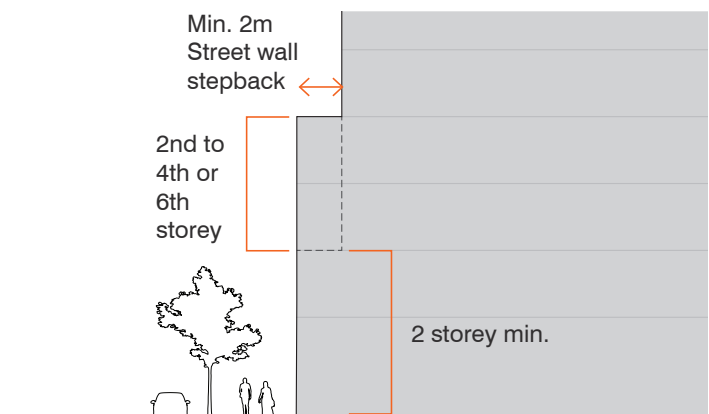
Diagram illustrating street wall height and stepback
