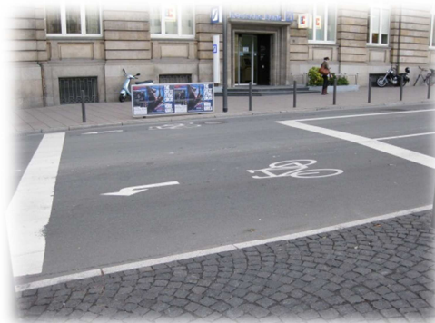
Bike boxes provide advance stop lines for cyclists to make left turns
