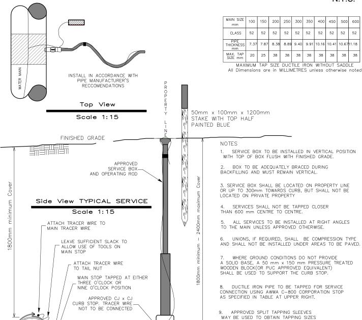
WATER SERVICES INSTALLED ON PVC PIPE SHALL BE CONCRETE BLOCK EQUIPPED WITH SERVICE SADDLES AND /OR FACTORY MADE TEES
