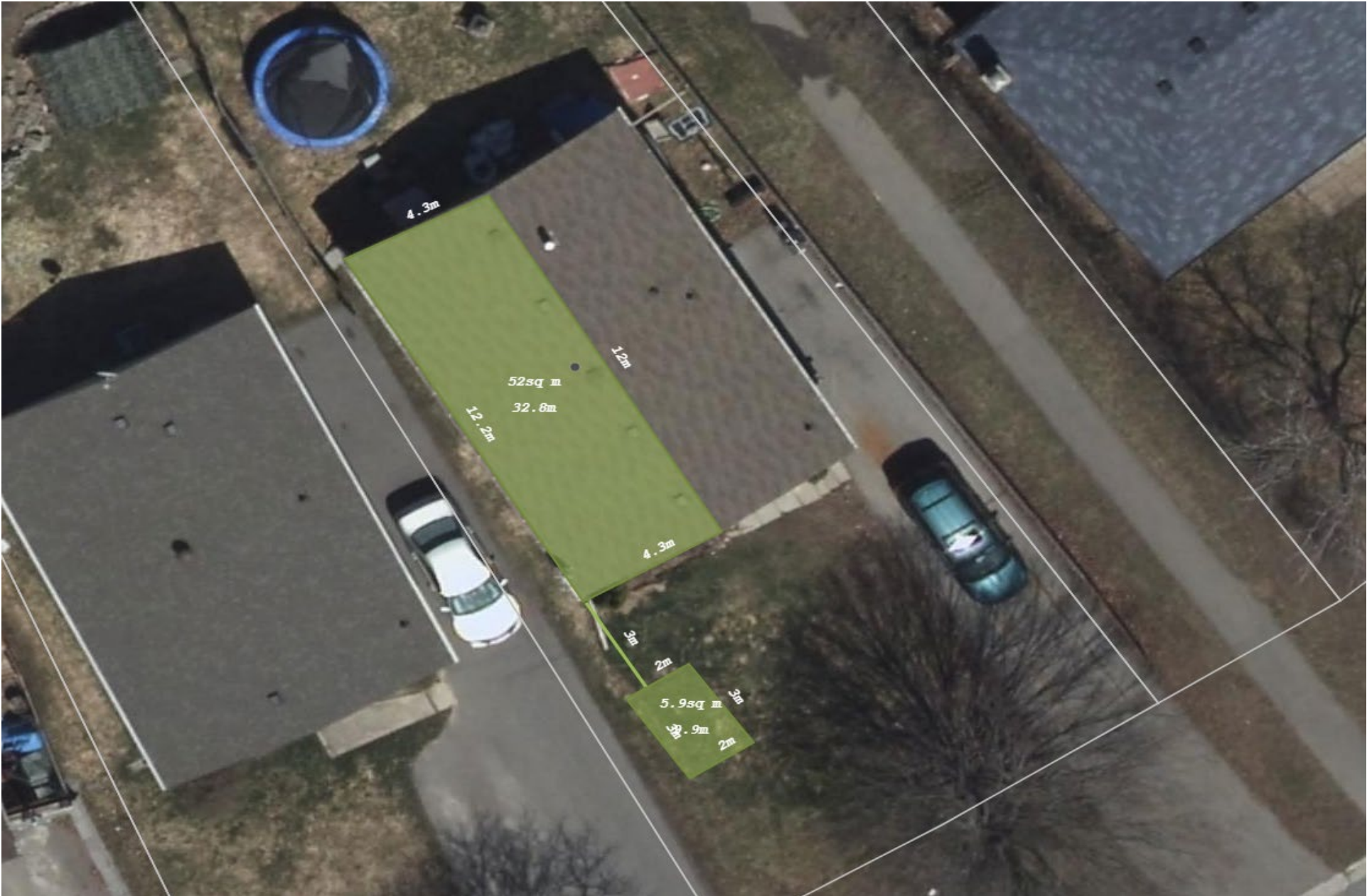
Figure 1: Complete aerial photo showing downspout locations, roof area, garden locations and all associated dimensions.
