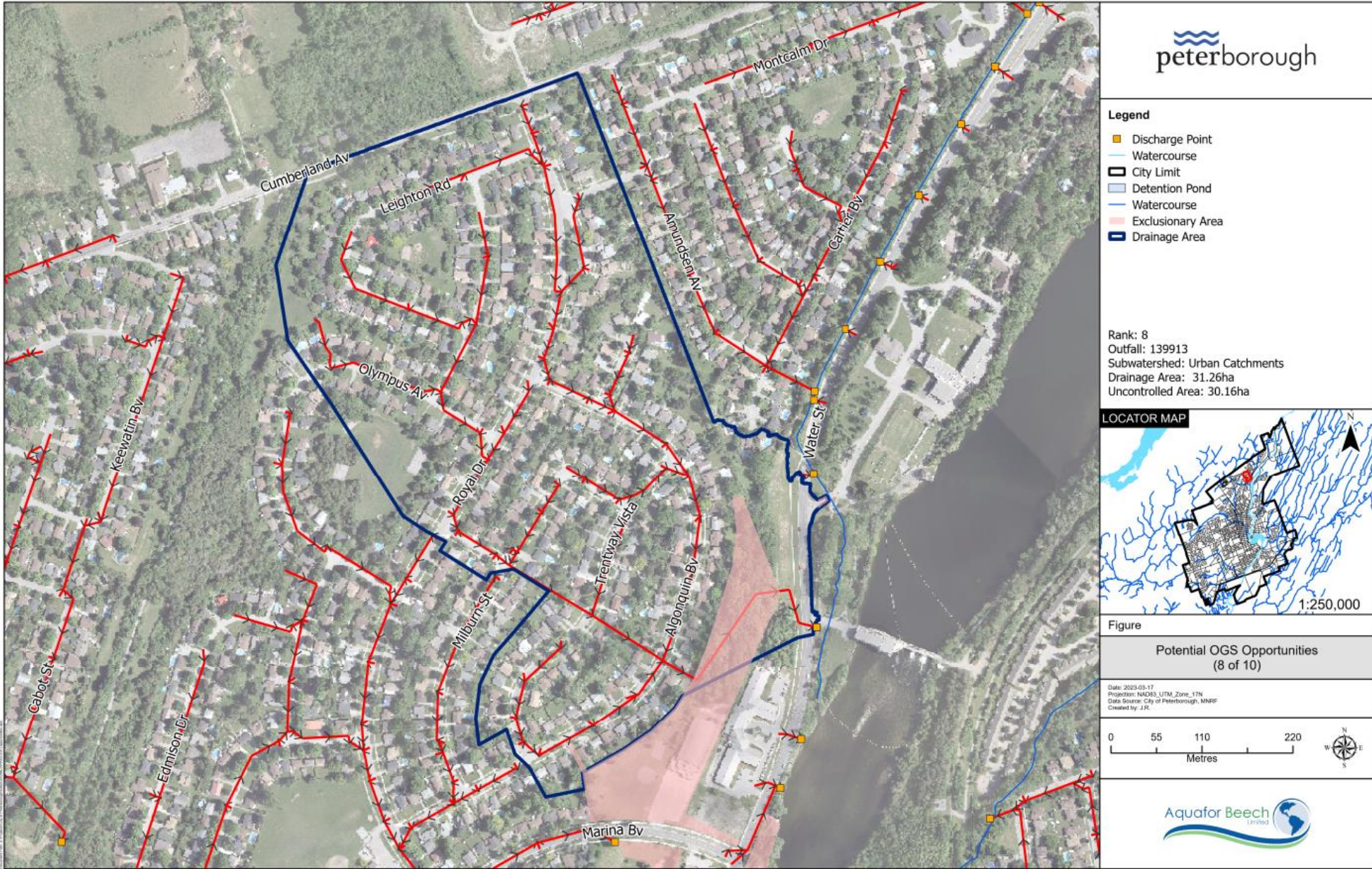
Figure 6-13: OGS retrofit location 8 and associated catchment
