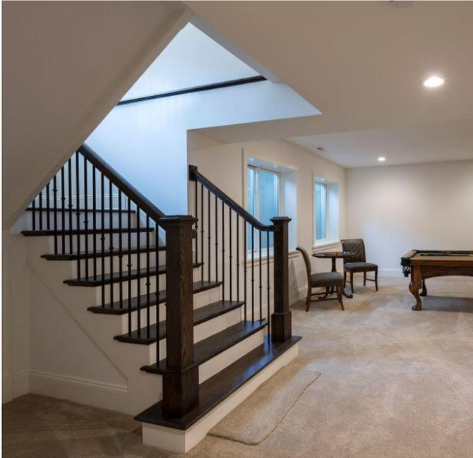
Stairs are required to have uniform riser heights within the flight of stairs (O.B.C. 9.8.). If you intend to raise the height of the finished floor, or if you intend to finish the stairs with flooring, uneven riser heights must be avoided throughout the entire stair run for safety reasons. Stairs must also contain a code compliant guard and handrail.
