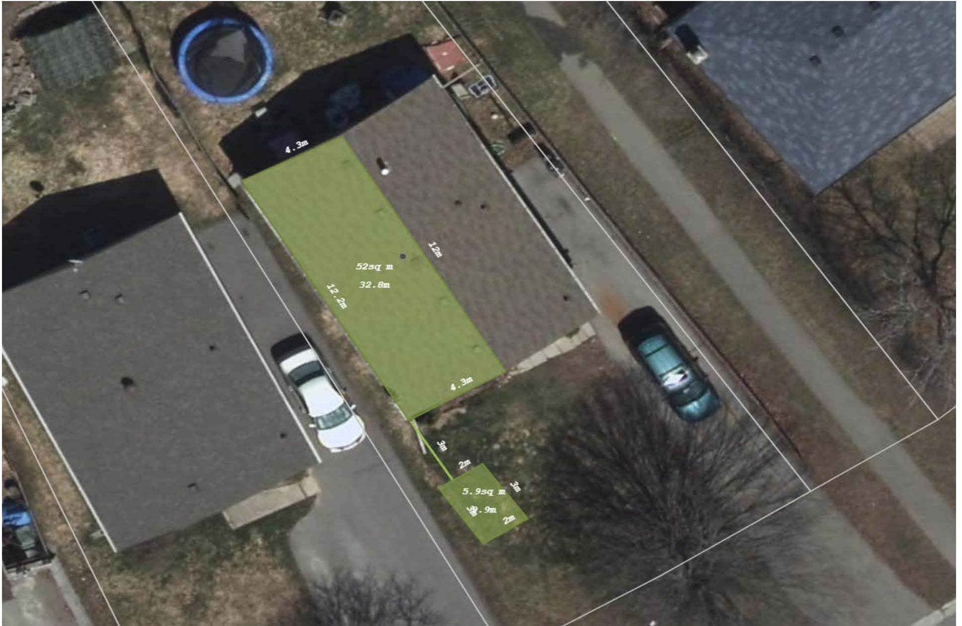
Figure 1: Complete aerial photo showing downspout locations, roof area, garden locations and all associated dimensions.
