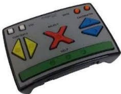
**Figure 1 – Audio Tactile Interface (ATI)**
